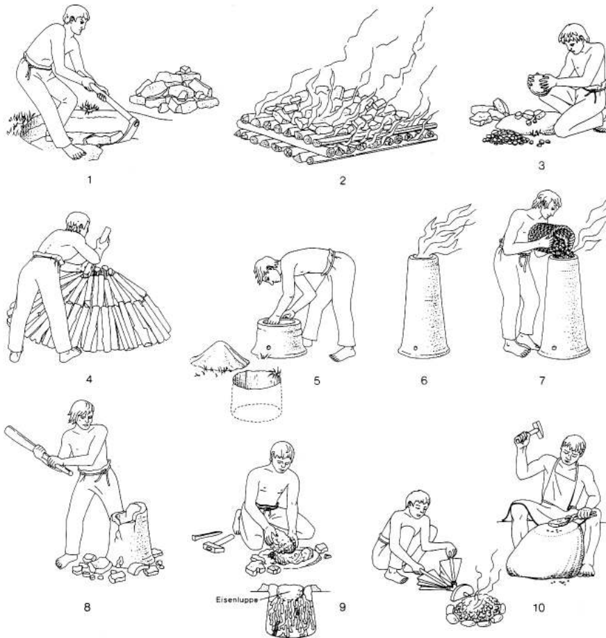
Fig. 1 Chaîne opératoire of the smelting of bog iron ore in the shaft furnace with slag pit. 1 – quarrying the bog iron ore; 2 and 3 – roasting and crushing the bog iron ore; 4 – charcoal production; 5 – construction of the shaft furnace above the previously dug out slag pit; 6 – pre-firing of the furnace shaft; 7 – filling the furnace initially with temporary filling material for the slag pit, then with charcoal and crushed iron bog ore; 8 – breaking the shaft furnace; 9 – removal of iron bloom; 10 – reforge the still hot iron bloom.
