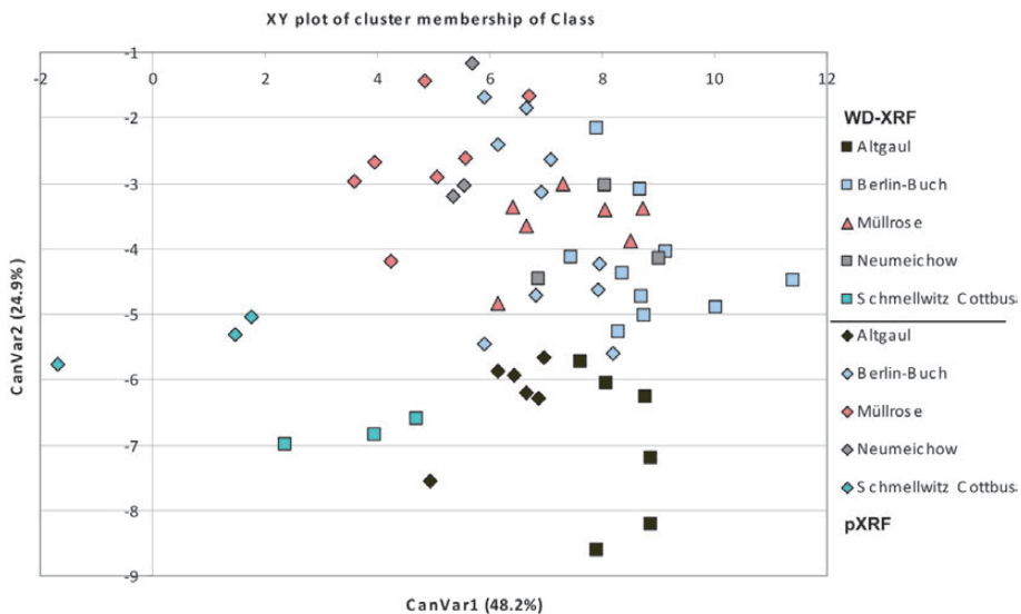
Fig. 5 Discriminant analysis of results by pXRF and WD-XRF for sherds of turban-edged pottery found at different sites in Brandenburg (elements used: Ti, Fe, Ca, K, Cr, Rb, Sr, Y, Zr, and Nb).
