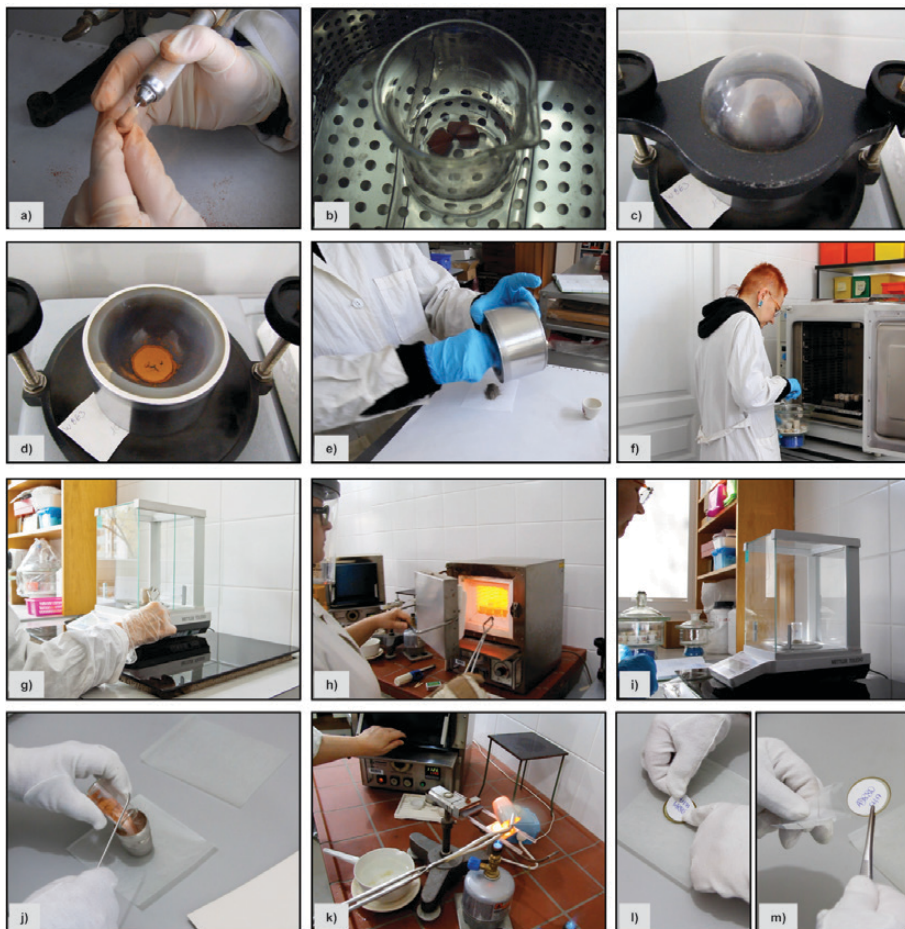
Fig. 6 Preparation of samples for WD-XRF analysis in the ARCHEA laboratory.
