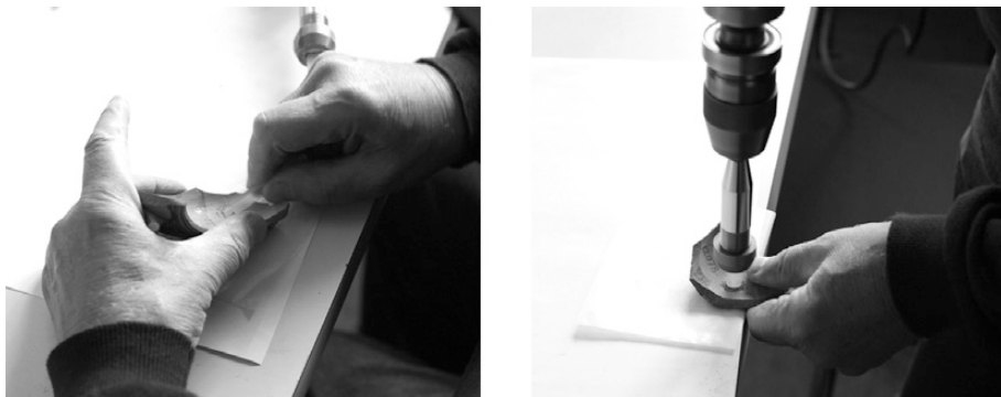
Fig. 1 Cleaning and extraction of sample by drilling.
