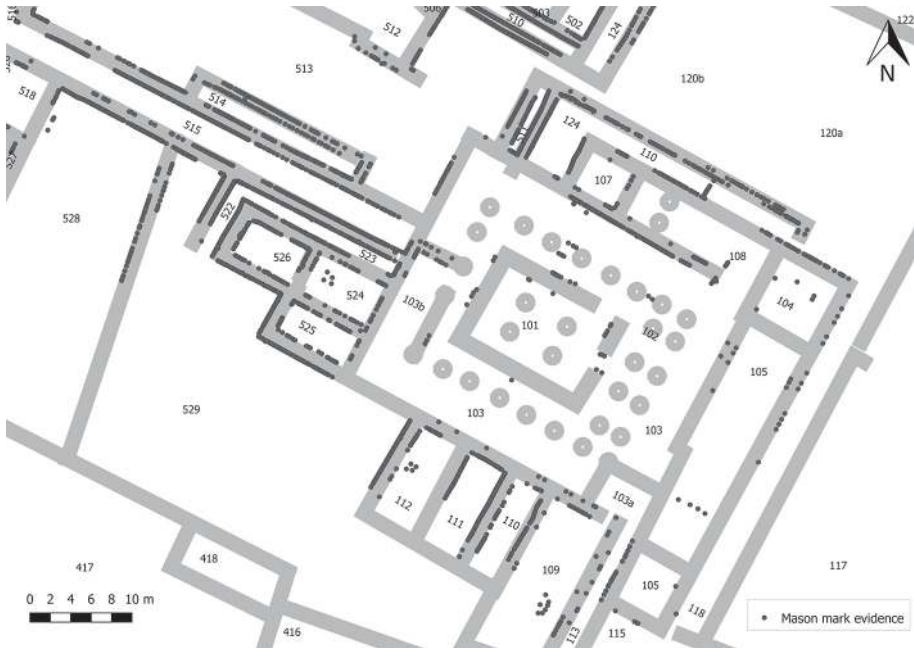
Fig. 17 Spatial distribution patterns of mason marks within central terrace complex of the Great Enclosure.
