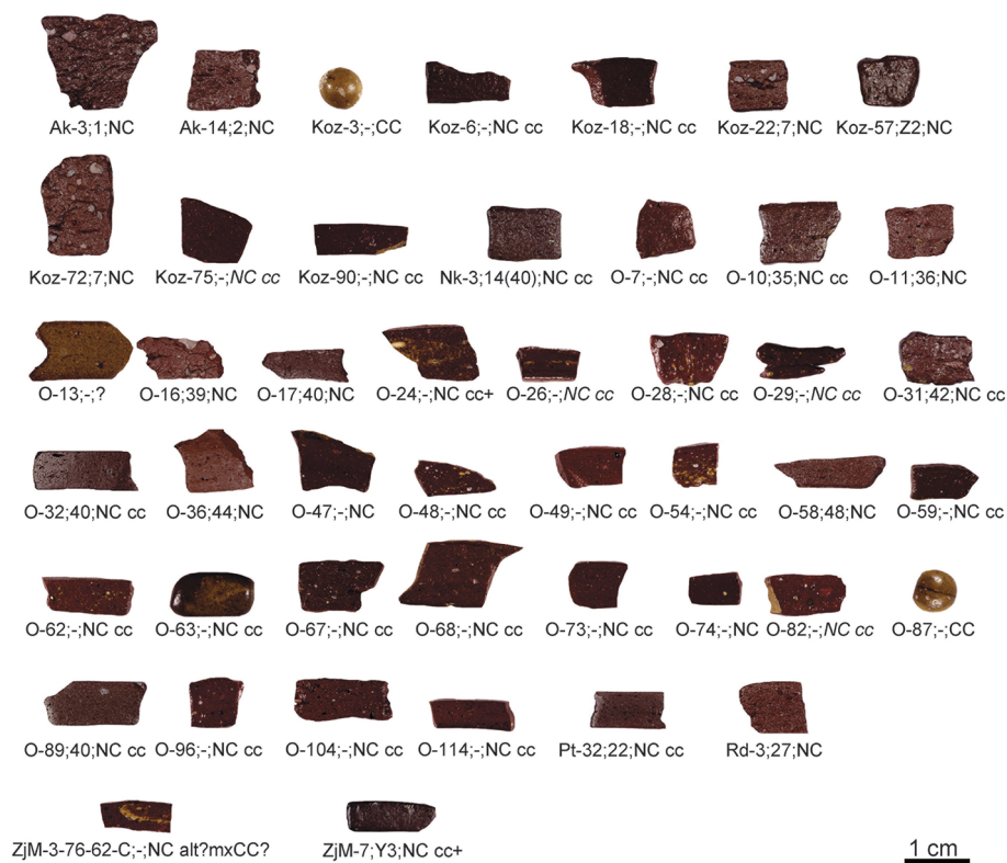
Fig. 23 Samples of cluster 1 arranged in order determined by cluster analysis of pXRF data. Samples (cut-sections) after refiring at 1150°C in air.
