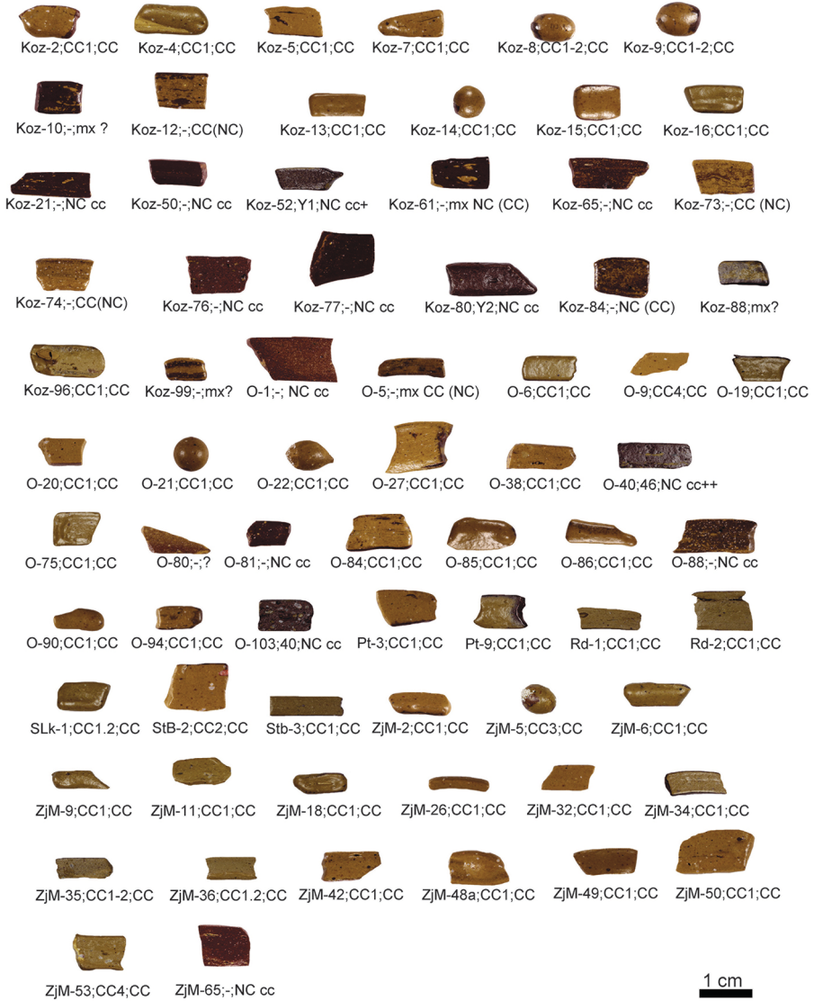
Fig. 24 Samples of cluster 2 arranged in order determined by cluster analysis of pXRF data. Samples (cut-sections) after refiring at 1150°C in air.
